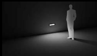
Location luminaire unshielded light
