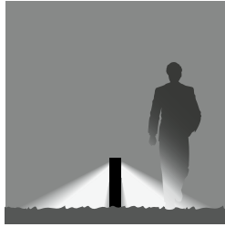
Height 600 mm: Symmetrical light distribution
